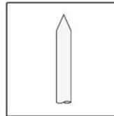
Smooth Pin type is designed for extremely sensitive merchandise, will not damage delicate fabric; the smooth type pin might be detached by spin and pull.
