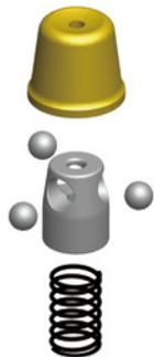
Ontime Company divides Super lock and Normal lock through the character of spring used in lock structure which is defined as bellow:
