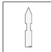
SuperTag Pin type is designed with a unique serrated pin shaft to function with SuperTag for securing a merchandise; the SuperTag pin might not be compatible for some extremely sensitive, delicate merchandise.
