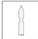
Serrated Pin type is designed with the improvement to deter the attempt of detaching the pin by spin and pull; the serrated pin might not be compatible for some extremely sensitive, delicate merchandise.
